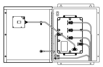
Figure 5: Three-Phase, 3-Wire, Delta Installation
