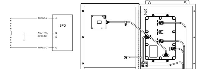
Figure 3: Three-Phase, 3- or 4-Wire, Grounded Wye Installation
