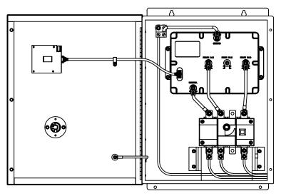
Figure 9: Three-Phase, 3- or 4-Wire, Grounded Wye Installation with Integral Disconnect
