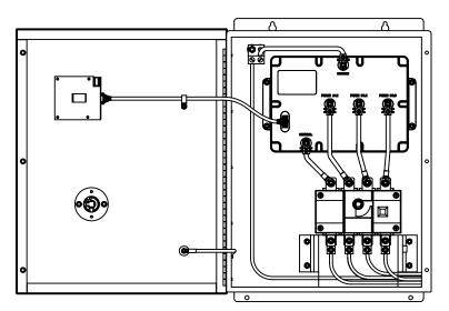
Figure 11: Three-Phase, 3-Wire, Delta Installation with Integral Disconnect
