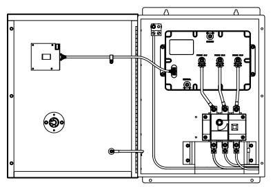
Figure 13: Three-Phase, 3-Wire, High-Resistance Grounded Delta Installation with Integral Disconnect
